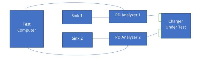
Some PD Analyzers, such as the GRL A1, can have multiple recording instances on one test machine as assumed in the setup shown above and the test procedure described below. Note that if the PD Analyzer used for testing needs one host machine for each PD Analyzer capture, such as for the Total Phase PD Analyzer, the test setup and procedure must be modified to include one Test Computer for each PD Analyzer.
