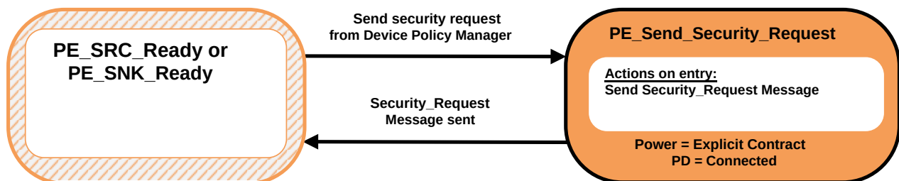
Figure 9.53. Send security Request State Diagram
