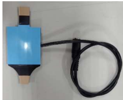
(b) Flexible Heater with Thermal Pad Attached on One End, and a Power Jack on the Other End
