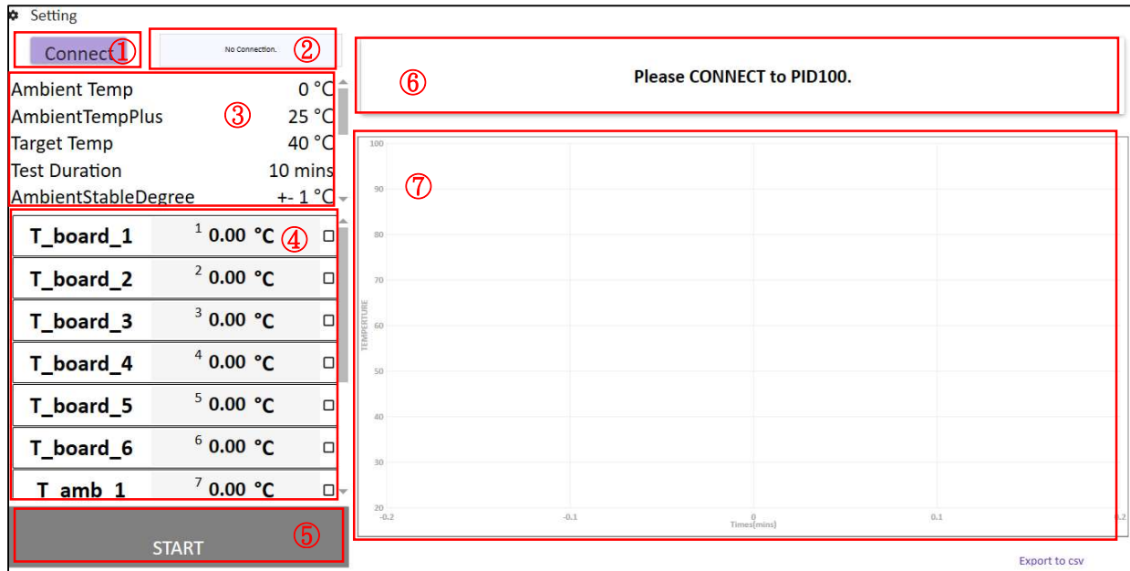
Figure 6 PID100 DAQ Software Interface
