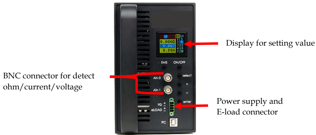
Figure 7 Power Delivery Source and E-load Unit
