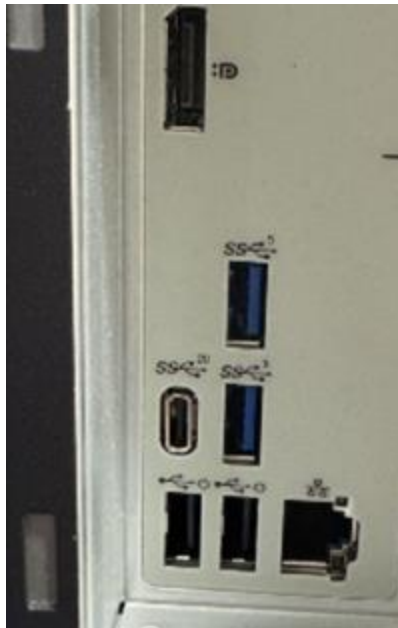
Figure 1: 5 Gbps and 20 Gbps Ports on Back Panel of XPS8940
