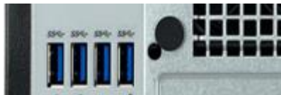
Figure 2: SS Ports on Back Panel of XPS8940
