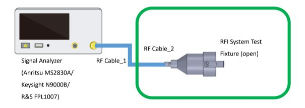
Start sweep and export data as CSV. Make sure that Noise floor does not exceed -105 dBm by making a graph with the data and setting the limit line.
