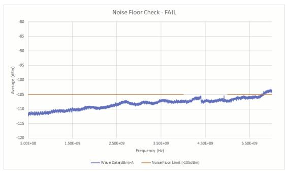
Below is an example of a failed Noise Floor measurement.
