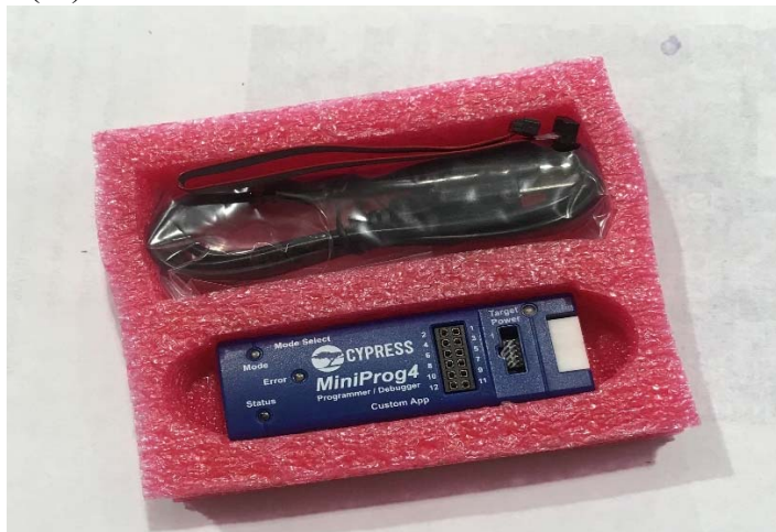
Figure 3: Cypress MiniProg4 Program and Debug Kit CY8CKIT – 005
