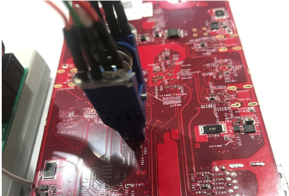
Figure 16: Connect the SPI flash component to UB10
